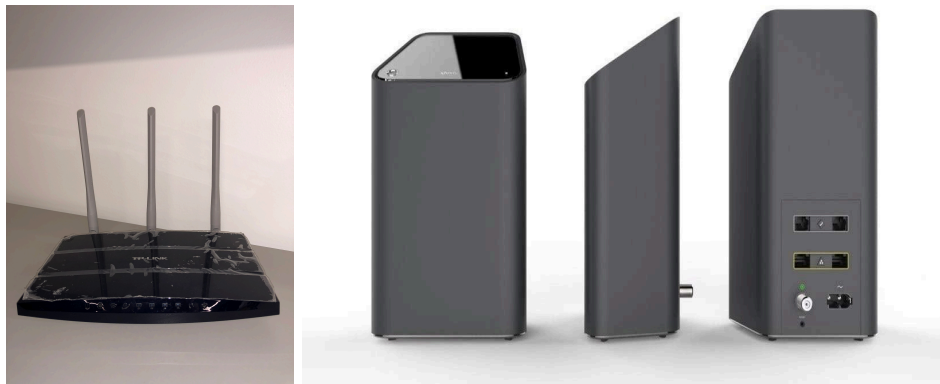
Figure 2. wireless router (left) and modem/router combo (right)
