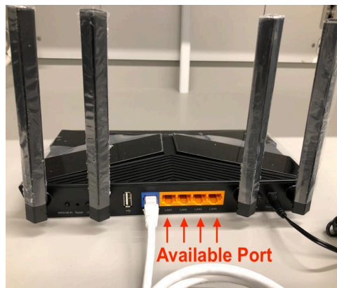
Figure 4. Available Ethernet ports on a wireless router
